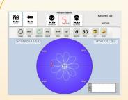
**Dynamic Test** offers a moving cursor that the user "follows". Four patterns are offered: Circle, Square, Infinity and Random. Each pattern is available in three dimensions: Small, Medium and Large; five speeds; Clockwise and Counterclockwise directions.
