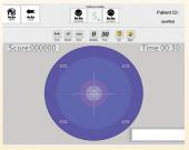
Static Test requires standing steady & balancing on the platform, keeping the crosshairs of cursor in the center of the test pattern. The Score indicates the deviation of user's center of gravity from the center of the pattern.
